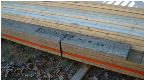
LVLs are built up of layers of veneer that are rotary-peeled from logs. These layers of veneer are coated with high-strength glue and stacked in a large billet to the desired length, width, and thickness. Usually, the grain in all of the layers is parallel. The LVL billet is cured in a heated press, which brings it to its final thickness
